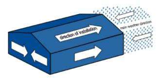
Horizontal installation of wall panels is performed bottom-up.
