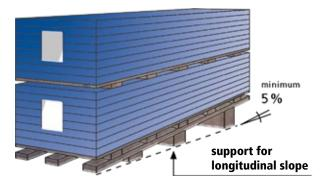
In case of storage of the packages directly on the roof, permission of the local site supervisor must be granted. Packages must be stored only on load-distributing support. Total load must not exceed the maximum load bearable by the support construction. Packages/panels are to be secured against gliding off. In case of interruption of installation work, open packages must be secured against wind exposure.
